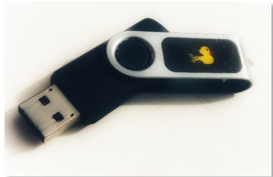
Figure 2: USB 'Ducky' acts as both keyboard and mass storage
